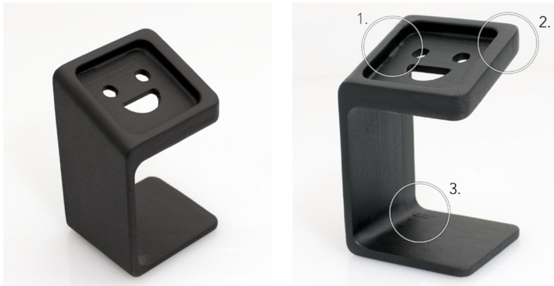
*A finished XTC-3D coated PLA part. **Circle 1:** Pooling of the XTC-3D has shown through the paint finish. **Circles 2 & 3:** Striations are still visible on the part.*
