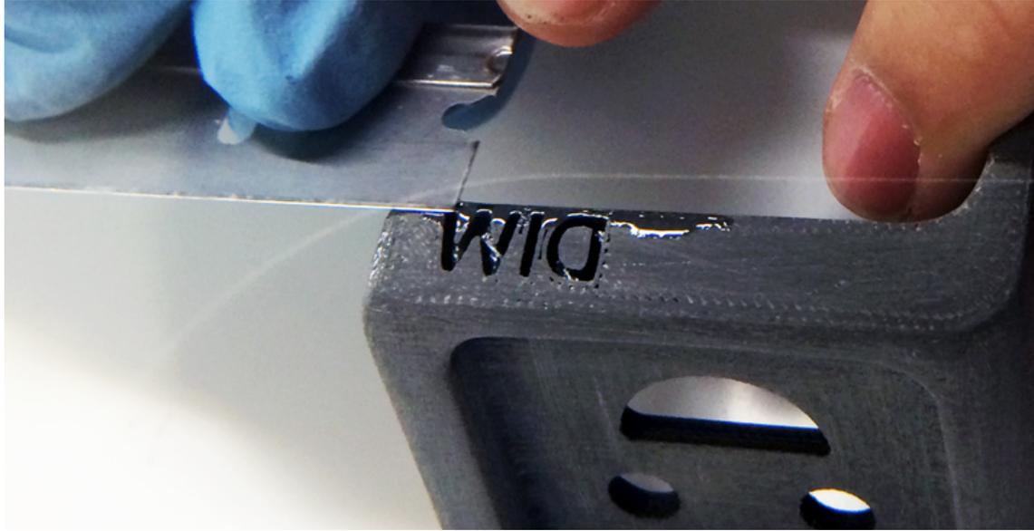
*Preparing the XTC-3D to fill the holes in the Dimension parts. A small amount of XTC-3D goes a long way: 12 grams was more than enough to repair the holes in the Dimension print and completely cover another PLA model.*
