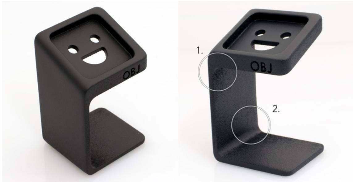
*A finished VeroBlack part. **Circle 1:** Notice how areas where the residue was not properly removed have a powdery paint finish. **Circle 2:** Faint stepping is visible in the paint finish, but for the most part starting with a smooth part has resulted in a smooth paint finish.*
