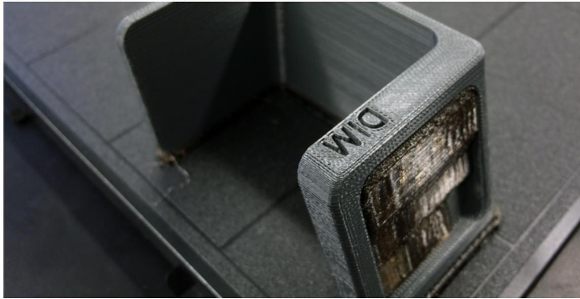
There are, however, clear stepping lines between the printed layers. If we don't remove these stepping lines, they'll show up in the final paint coat which will ruin our smooth finish. Thankfully, removing these will be easy thanks to ABS's high melting point and easy sandability.
