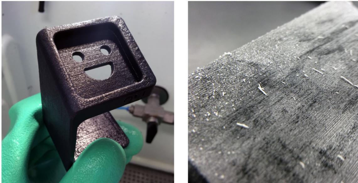
***Left:** freshly cleaned VeroBlack part out of bath after support material removal. **Right:** After drying there will still be trace amounts of residue which will fall off in small soft white chunks with dry sanding at around 100 to 300 grit.*
