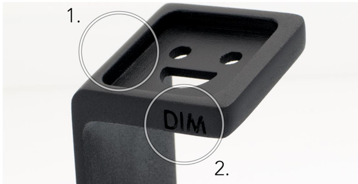
*The finished ABS part. Notice stepping is still visible on sharp internal geometry at Circle 1. but the holes around the DIM are not visible in the paint coat at Circle 2.*
