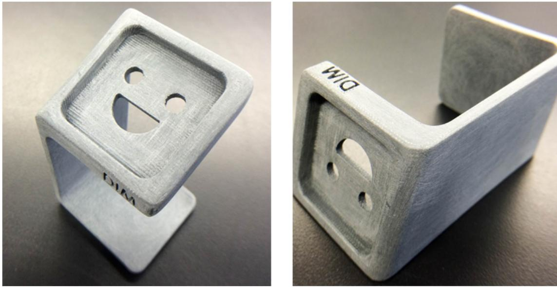
*A sanded and repaired ABS print. Note that the some layers are still apparent on difficult-to-sand internal corners.*
