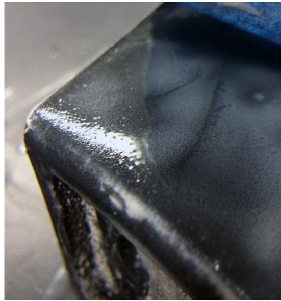
***Left:** Removing the residue will reveal a harder surface that we can paint on. **Right:** Wet sanding through 600 grit to remove the residual layer is very effective, thanks to the Objet's water soluble support material.*
