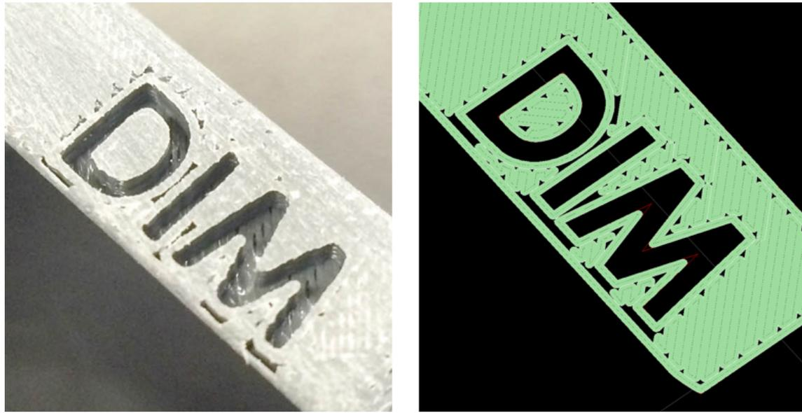
*Sanding reveals the holes left by the incomplete layer and are represented in Catalyst, where black shows lacking toolpaths in the top layer.*
